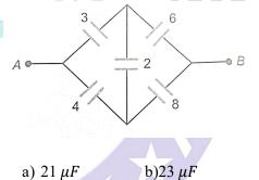
9. In the figure shown the equivalent capacitance between A and B is:
