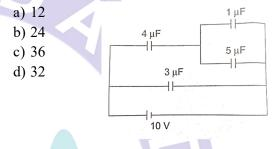
8. Effective capacitance between A and B in the the figure shown is (all capacitance are in  $\mu F$ )
